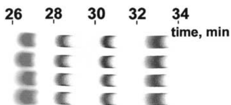
Figure 8. Four-channel fully on-line OPLC separation of dyes collected in parallel by chromatographic paper at outlets using FEW for segmentation. External pressure, 5 MPa; flow rate, 500 \mu\text{L}/\text{min} ; eluent, methylene chloride; 250 \mu\text{L} injection for four parallel channels; speed of chromatographic paper, 50 mm/min.
